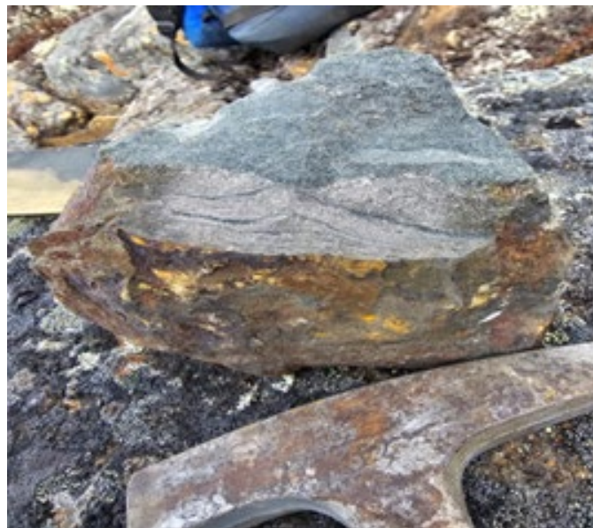
Figure 2 - Ultramafic/Massive Cu Ni Pt Pd sulfides contact in boulder, Blue Lake North
